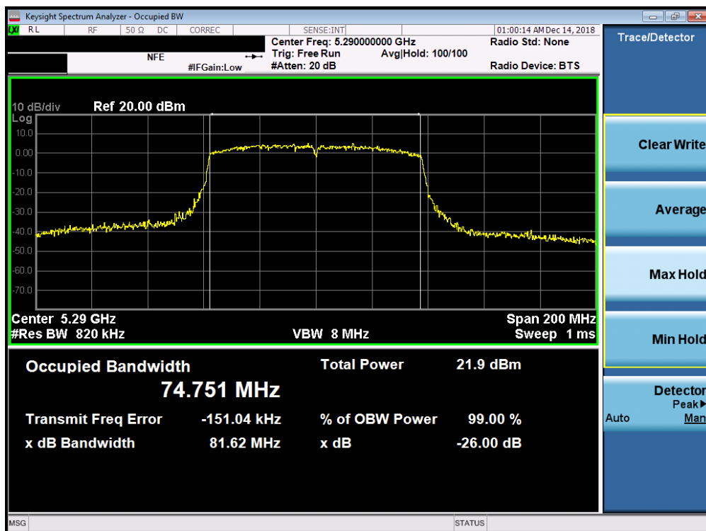
Plot 7-48. 26dB Bandwidth Plot SISO ANT2 (80MHz BW 802.11ac (UNII Band 2A) – Ch. 58)
