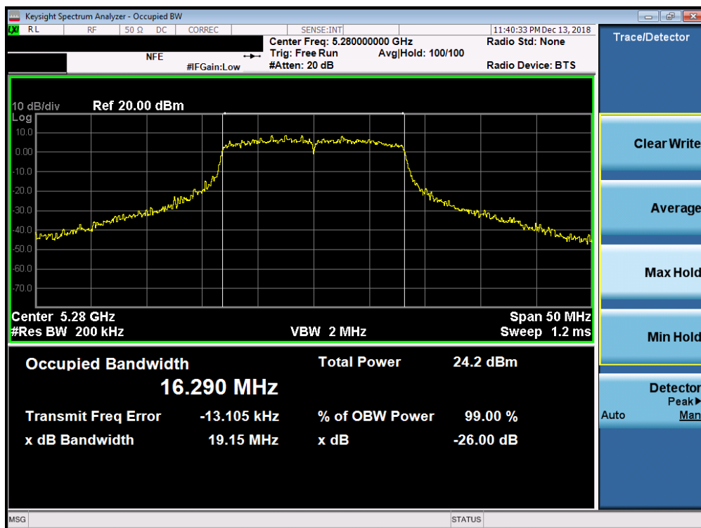
Plot 7-11. 26dB Bandwidth Plot SISO ANT1 (802.11a (UNII Band 2A) – Ch. 56)
