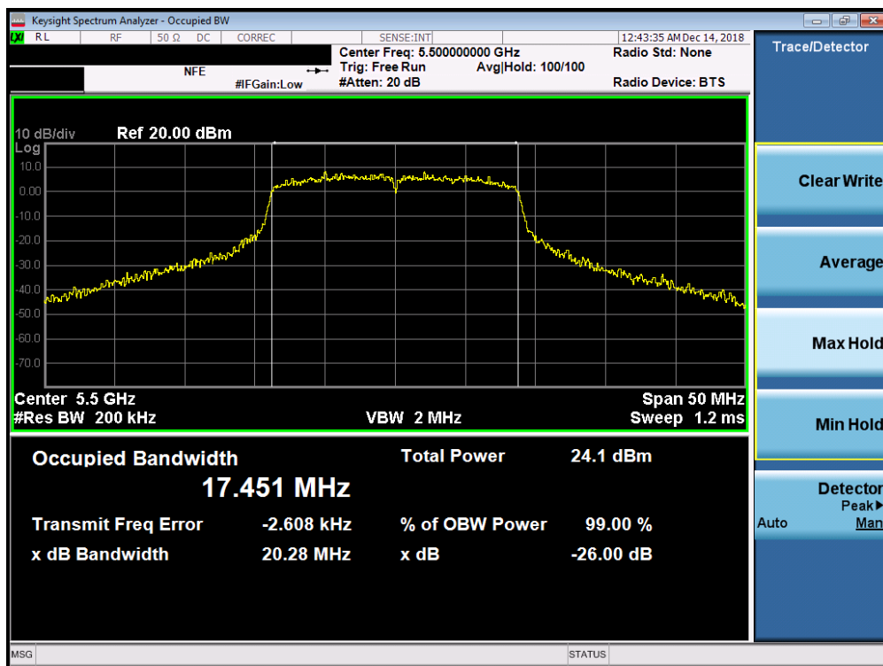
Plot 7-52. 26dB Bandwidth Plot SISO ANT2 (20MHz BW 802.11n (UNII Band 2C) – Ch. 100)
