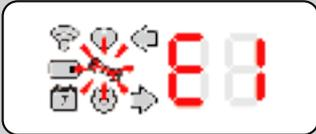
There are temperature sensors that sit above each CO<sub>2</sub> canister. When the canister discharges the temperature drops and this is detected by the Radar X, if this temperature drop is not seen this error will be raised. Possible causes of seeing this error are:
