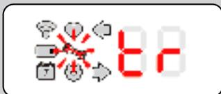
The unit triggered due to the sensors detecting activity, there were no issues detected in activation. This is the "normal" indicator that the Radar X has trapped and everything is okay.
