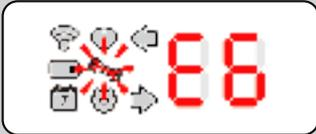
Not deployed, unit could not self deploy or was not service correctly. **Both** catch sides of the unit are in a state that renders the unit non functional. This could be door not closed properly, trigger pin not set - or combination of these, see E0 above.
