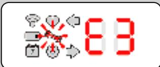
The unit triggered its CO<sub>2</sub> due to a heavy impact. Possible causes of seeing this error are:
