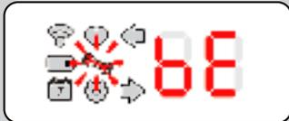
The unit is currently designed for 3 wire alkaline batteries. The packs used have a method of reporting to Radar X what battery technology has been fitted. If for some reason this can't occur then the unit is unable to calculate the battery %. This could be caused by using a pack not supplied by Rentokil, or a damaged battery lead or to the battery itself. The unit may still operate, but you should consider replacing the battery pack.
