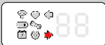
Eg: Right motor fired, double bar indicating armed pin on right side removed.
