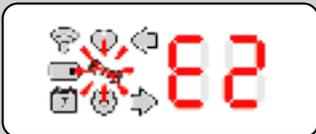
The CO<sub>2</sub> canisters are rated at a temperature of up to 50°C. After which they run the risk of rupture. The Radar X will prevent this by triggering prior to reaching the upper threshold of 50°C. You should survey the installed area to ensure that the unit is not placed in an area that gets to these temperatures.
