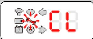
It has been detected that the sensor enabling the unit to detect mice has reduced capability for some reason. For an IR sensor pod, this means that one or both of the sensors within the pod are reading below what they should. For IR sensor pod this could be due to:
