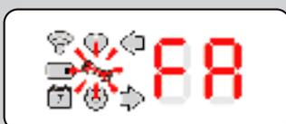
If a unit is detected as non functional such as continual “CL” on both sides or a Manual test shows the unit is still faulty, then you will see this error and the unit **must** be decommissioned from site and CO<sub>2</sub> canisters and battery removed.
