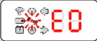
Manual pod test not passed - replace pod.
