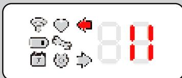
Eg: Left motor fired, double bar indicating armed pin on left side removed.
