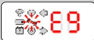
Sensor pod has failed. It **must** be replaced. The damage might have occurred due to moisture ingress, scratched/damaged lens, no feedback from one or both of the IR's within the sensor pod.
