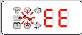
The battery is too low or too high a voltage to reliably run the system in the environment for which it is specified. You must replace the battery pack.
