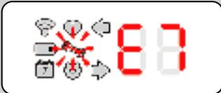
The unit has been disabled from triggering remotely by the server, you will only ever see this on a Connect Radar X. You can service it and it will be rearmed and operational, however you should understand why it might have been deactivated remotely in the first instance before doing this.
