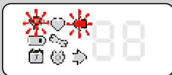
First tap in LED Test Mode. All icon and diget segments are turned off. Left arrow (Icon
