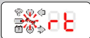
The unit was triggered remotely by the server, you will only ever see this on a Connect Radar X. You can service it and it will be rearmed and operational, however you should understand why it might have been activated triggered remotely in the first instance before doing this.
