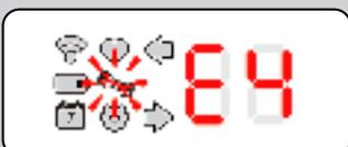
The unit moved/sustained a shock which didn't cause it to trigger, but it may not be positioned where it should so you should check the floor plan app, as well as inspect it for damage as in E3 above; the unit must be Serviced and inspected for damage/cracks/chips.
