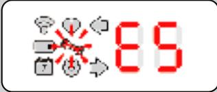
The trigger pin has not been locked in place. You may have armed the red doors, but failed to move the trigger pin into the locked armed position. Go back into Service mode and you must arm the trigger pin.
