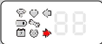
The right arrow (Icon
