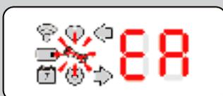
There was an issue with the trigger mechanism, this code will allow you to go into a tech mode that allows you to trigger the unit using the service key. Before doing this read and understand the section “Manual Trigger Testing” as it involves moving parts and potentially CO<sub>2</sub> escaping with the catch trays open.
