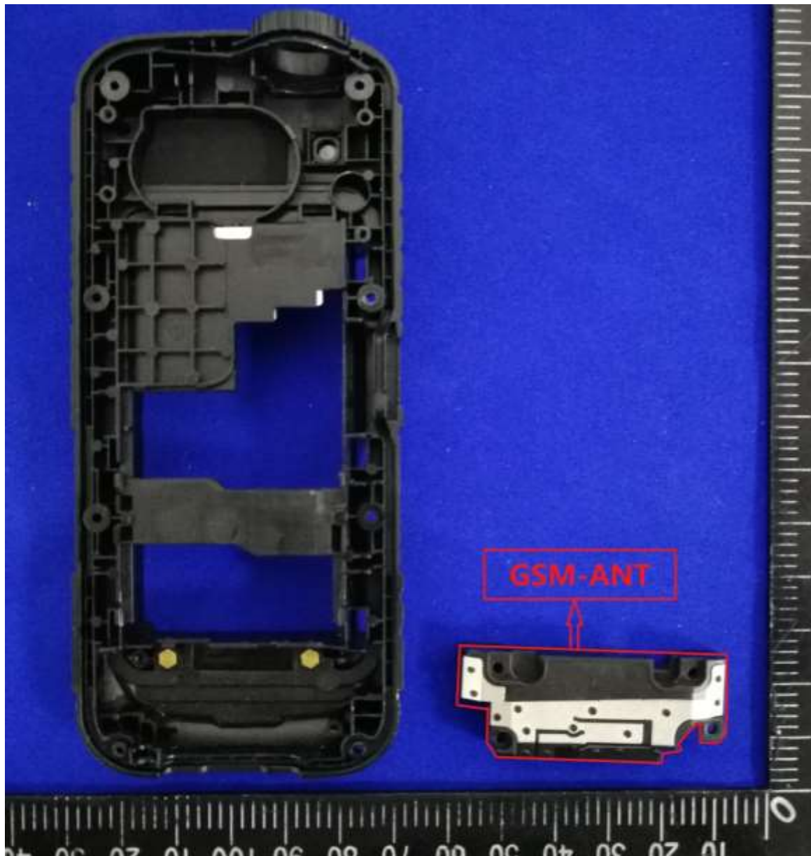
Fig.14.1 EUT Antenna Locations
