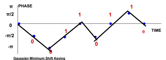
MSK has high sidebands relative to the main lobes in the frequency domain - this can lead to interference with adjacent signals.
