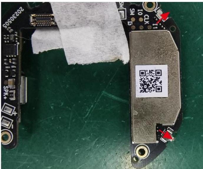
At present, the antenna uses these two shrapnel, matching series 0 ohm, ground empty paste
