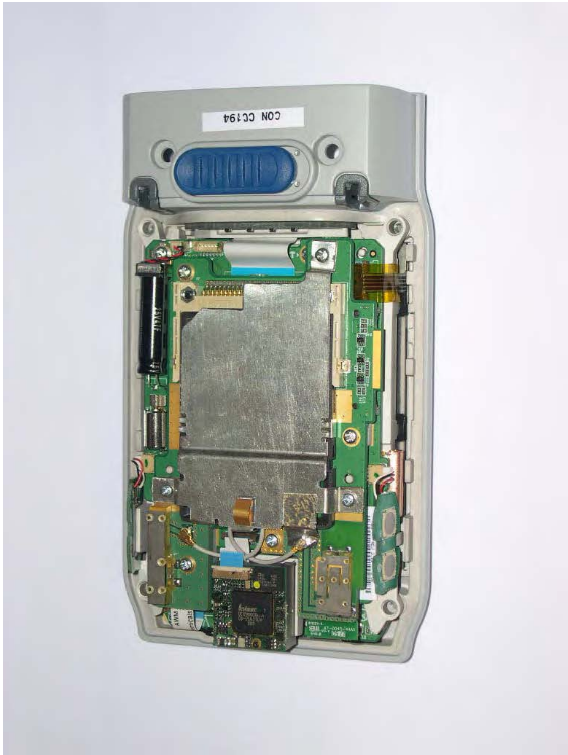
CN30 Console Internal View
