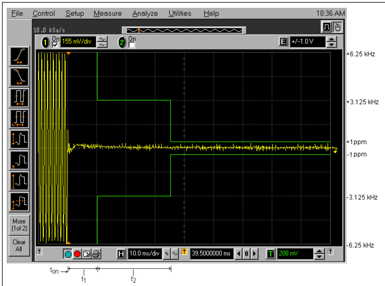
Plot 5.8.4.5. Transient Frequency Behavior for 6.25 kHz Channel Spacing 406.2 MHz, High Power Setting, Switch on condition t_{on} , t_1 , and t_2
