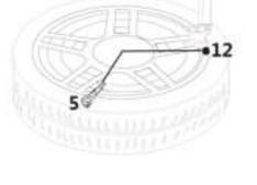
1.8 Dynamically balance the wheel before it is placed back on the vehicle.
