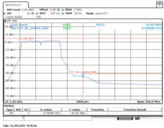
MIMO A, 802.11n20, HT8, CH62, BE High RMS
