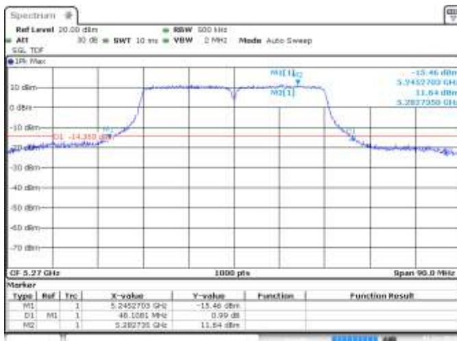
SISO B, CH54, 802.11n40, HT0, 26dB BW
