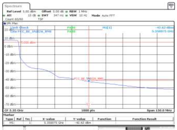
SISO A, 802.11n40, HT0, CH62, BE High RMS
