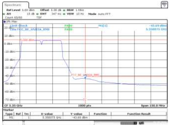
SISO A, 802.11n40, HT0, CH54, BE High RMS
