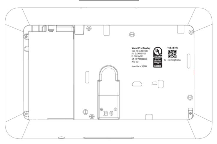
Note: The label is permanently laser etched on the back cover of the product.
