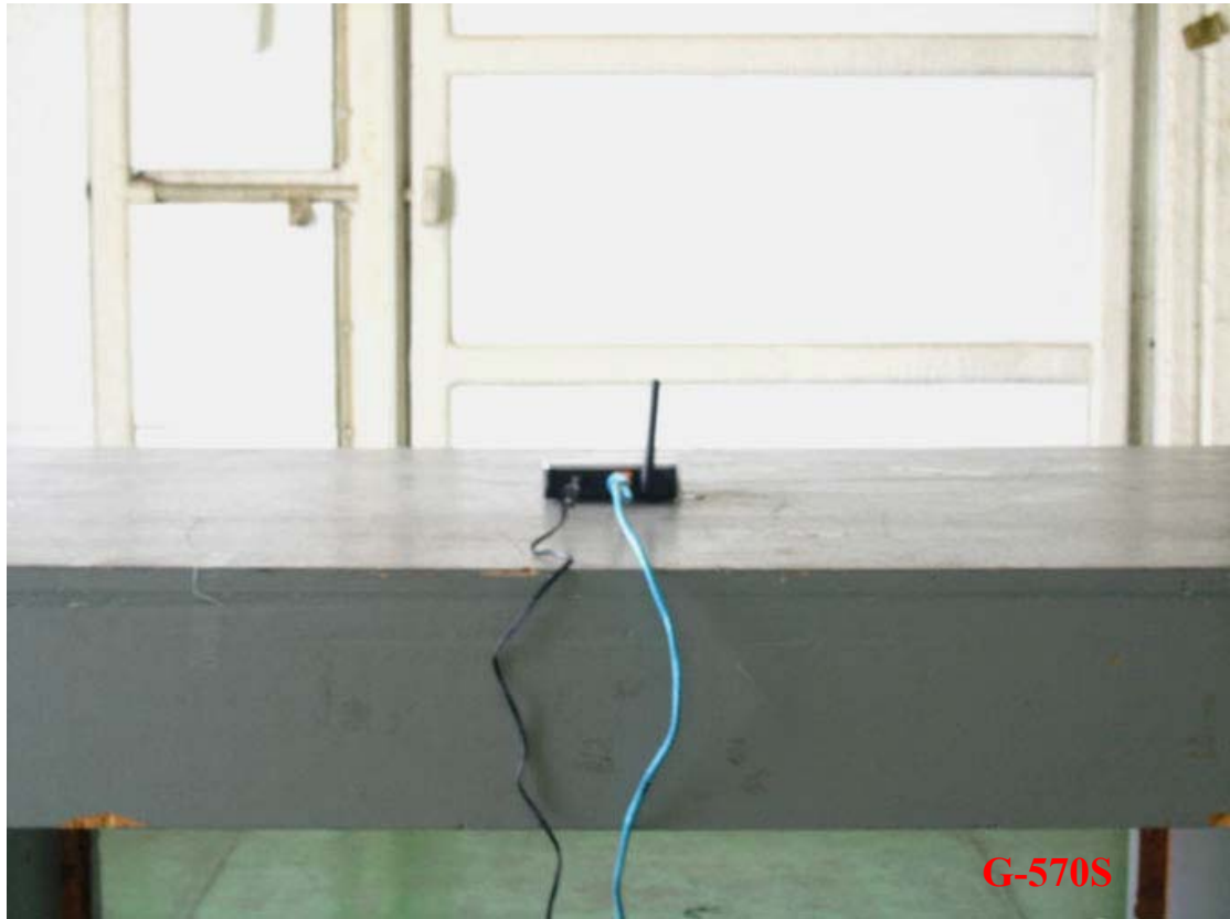
Photo 2: Radiated Emission Test set-up photo
