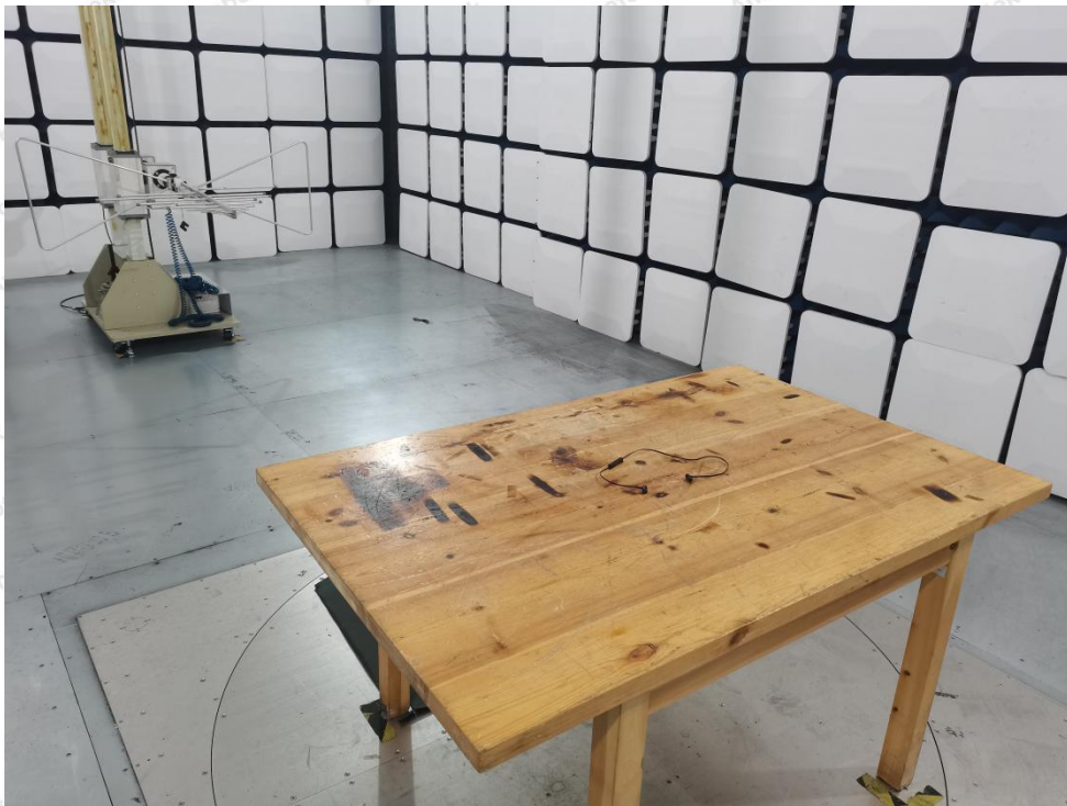
Photo of Radiation Emission Test
