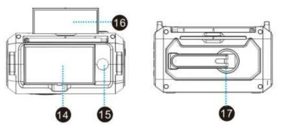
**Solar charging panel:** Align the solar panel with sunlight and it will automatically charge the device. The orange indicator light on the display screen will be on when the solar panel is charging the device.
