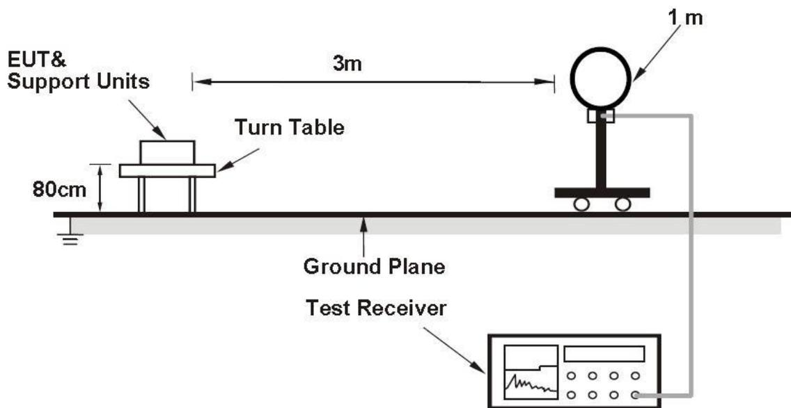
For Radiated emission 30MHz to 1GHz
