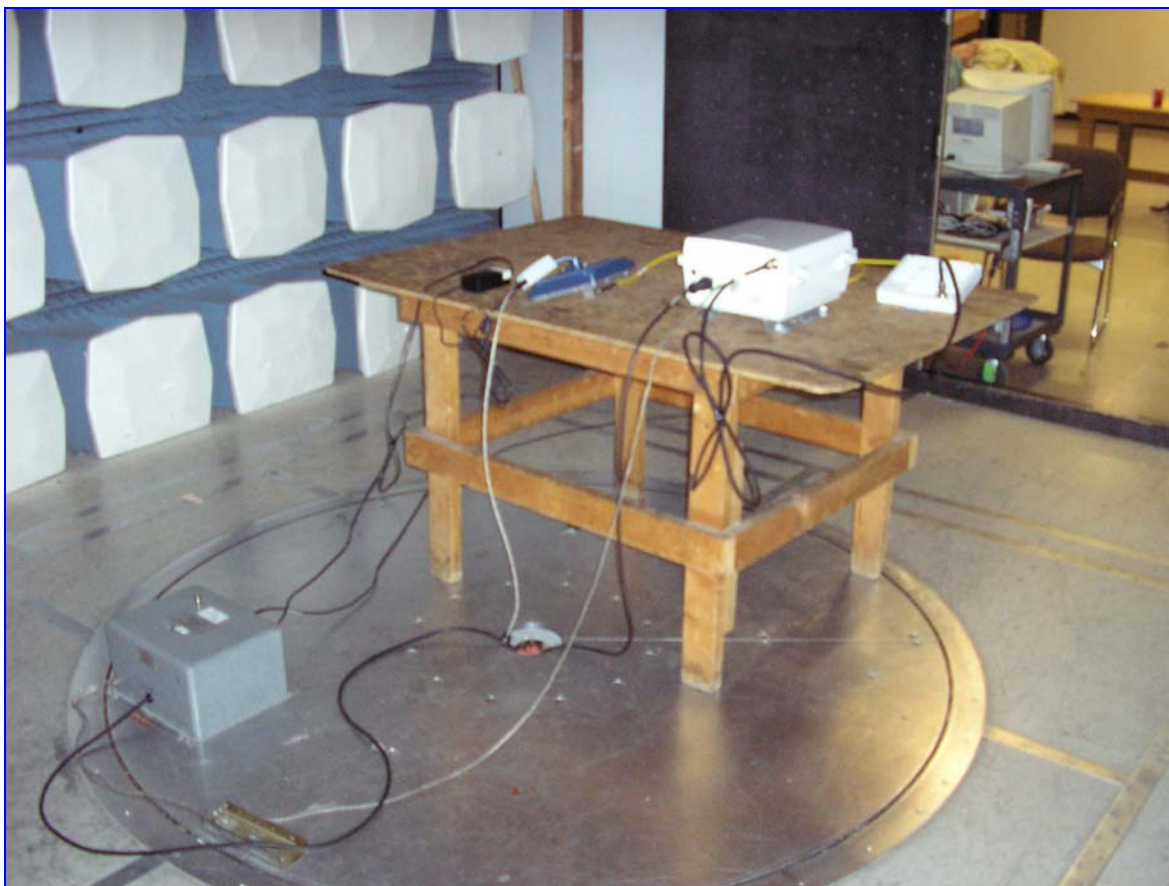
Photograph 1. Conducted Emissions Test Setup
