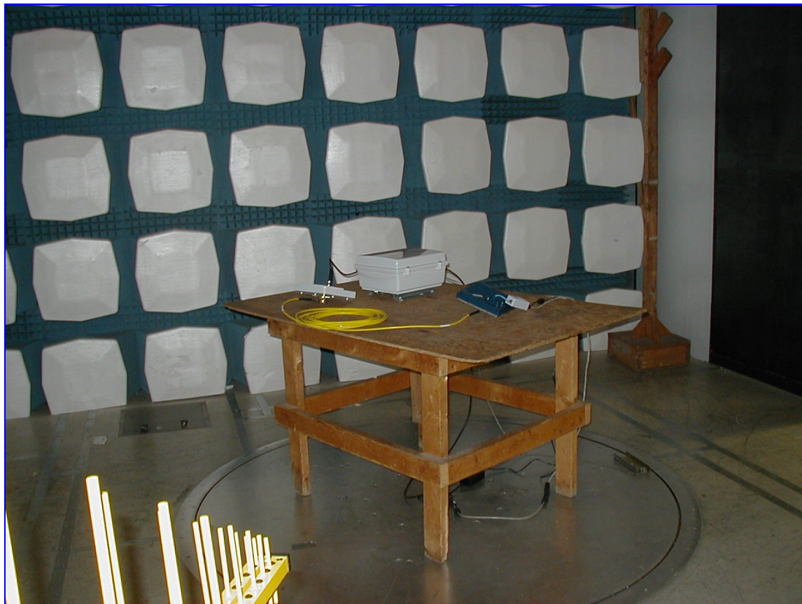
Photograph 3. Radiated Emission Limits Test Setup
