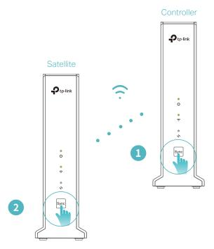
The Sync LEDs of the Controller and the Satellite light green and turn off about two minutes later. The Wireless LEDs of the Controller and the Satellite should be solid green after successful synchronization.
