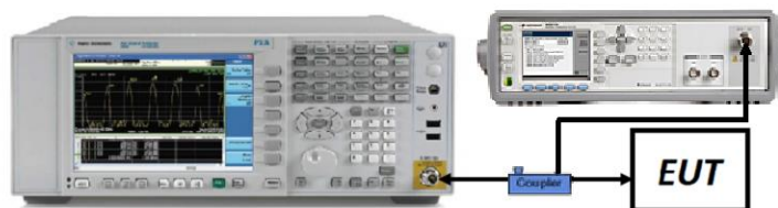
Figure 7-5. Test Instrument & Measurement Setup
