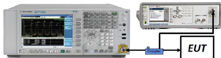
Figure 7-3. Test Instrument & Measurement Setup
