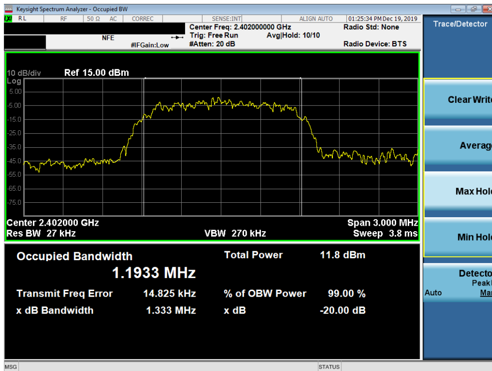
Plot 7-4. 20dB Bandwidth Plot (Bluetooth, 2Mbps – Ch. 0)
