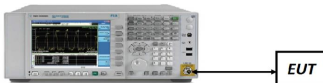
Figure 7-3. Test Instrument & Measurement Setup
