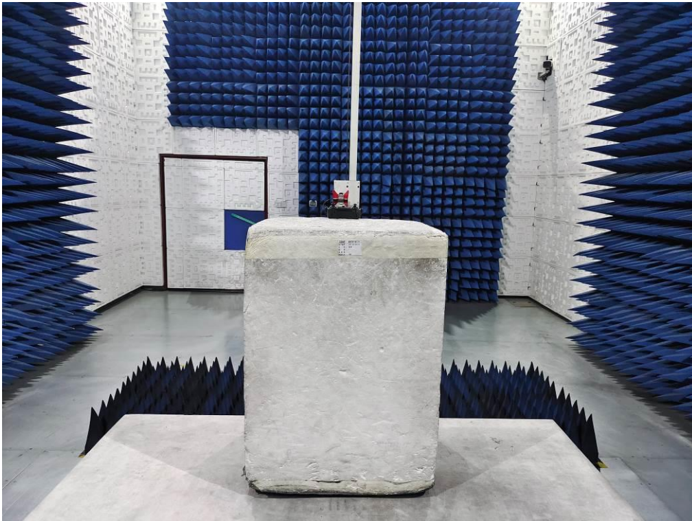
FCC RADIATED EMISSION TEST SETUP ABOVE 1GHZ
