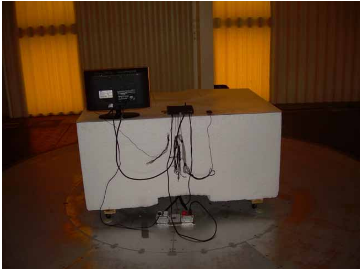
Photograph 3 - Back View Radiated Disturbance Configuration – Cirocomm Technology Antenna
