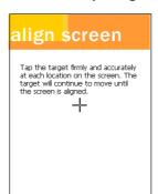
Use the stylus to tap the center of the target (+ sign). The target moves each time you tap it, the adjustment ends after you tap it five times.
