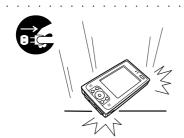
Should you drop Rugged PDA and damage it, immediately shut down the power and unplug the AC adaptor from the power outlet. Continued use creates the danger of shorting, fire and electric shock.
