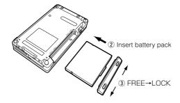
Be sure to slide the battery pack cover lock switch to the LOCK position. If it is not attached correctly, it may fall out while you are carrying the Rugged PDA and cause a malfunction or injury.
