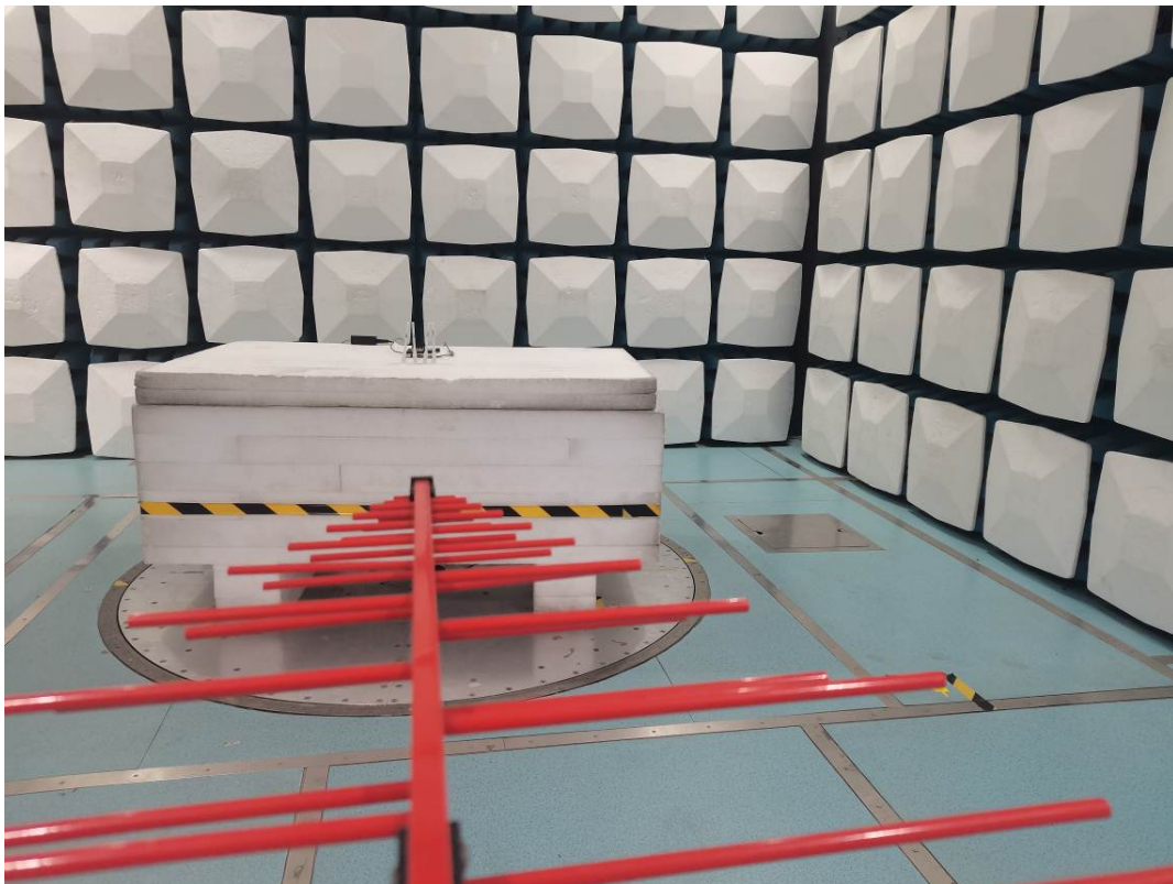
Radiated Emission 30M-1GHz View
