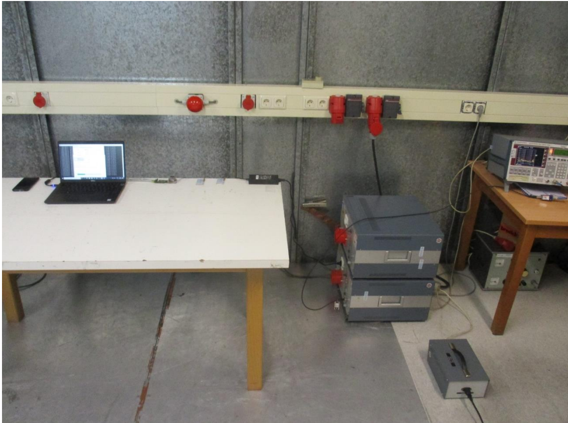
Photo 4 Photograph conducted emissions 0.15-30 MHz
