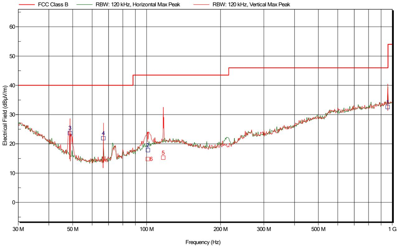
Figure 6.4.7.1: Electric field emissions Plot, 30MHz to 1GHz
