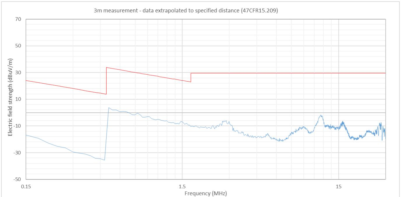
Figure 6.3.8.4 : Magnetic field emissions Plot, 150kHz to 30MHz Perpendicular orientation
