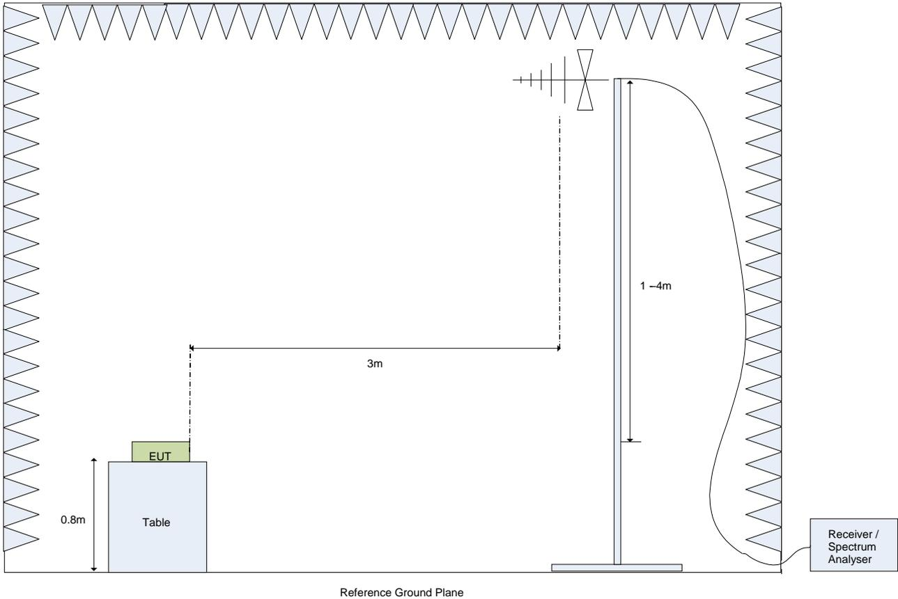
Figure 6.4.6.1: Test Setup for E-Field Measurements from 30MHz to 1GHz
