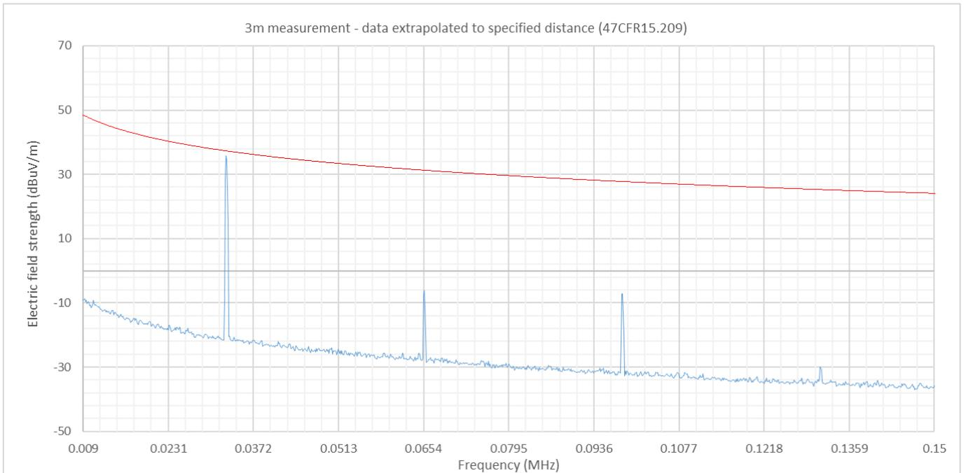
Figure 6.3.8.2: Magnetic field emissions Plot, 9kHz to 150kHz Perpendicular
