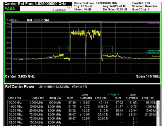
Middle Band Edge, 2 Carrier, Modulation: 16QAM, BW=15MHz
