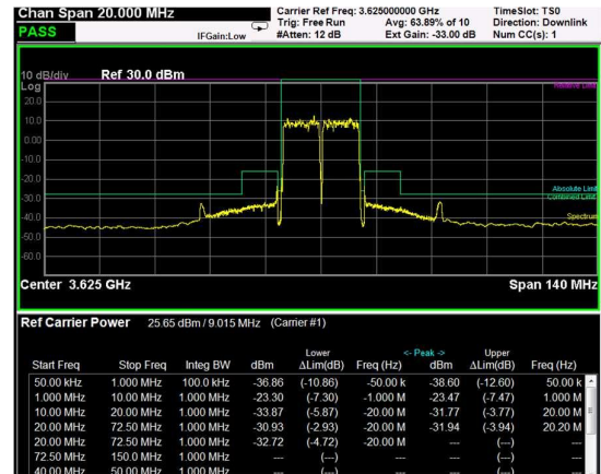
Middle Band Edge, 2 Carrier, Modulation: QPSK, BW=10MHz
