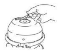
Remove the release stud assembly from the side pocket, and remove the release nut and washer from the release stud.
