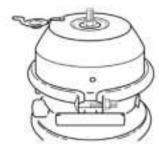
S. With a wrench, turn the release stud assembly nut until the compression spring is 90-95 percent caged. While doing this, make sure that the pushrod (adapter pushrod, or service pushrod) is retracting. DO NOT over-torque the release stud assembly. (S-cam-type maximum: 50 lb-ft (68 N·m), Wedge-type maximum: 30 lb-ft (41 N·m)). The spring brake is now mechanically released.
