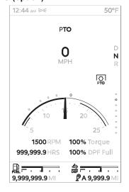
This truck may be equipped with Power Take-Off (PTO). PTO operation is enabled by using the dash mounted PTO switch in conjunction with the Cruise Control controls.
