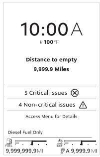
Post Trip presents information the driver might require for the next time the vehicle is operated, such as active warnings and the distance to empty. Post trip is shown when the ignition switch is turned to OFF. During Post Trip, the menu can be accessed by pressing **Select**.
