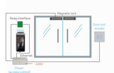
System installation schematic drawing for magnetic door
