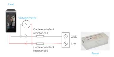
2. The power adapter with the device is shown as follow, 1m in total length, with 40cm low voltage power cable and 40cm high voltage power cable.
