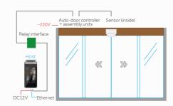
System installation schematic drawing for automatic door
