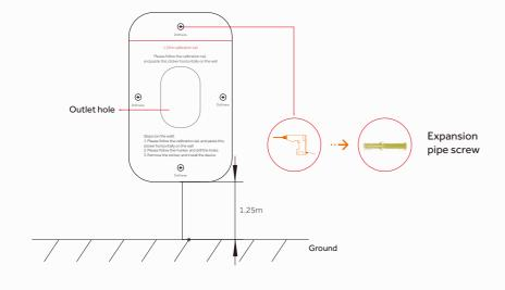
Move the support (device) to align the 4 holes on it with holes on the wall, and use the screws to fix the support (device) on the wall.
