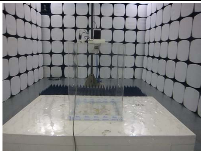
Radiated Spurious Emissions Test Setup Above 1GHz
