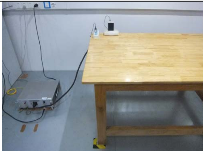
Conducted Emissions Test Setup Front View
