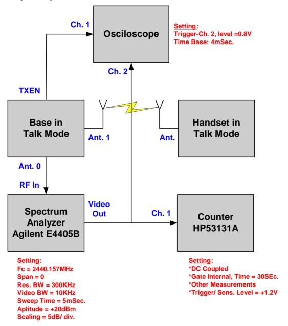
Step 1: Establish Single Channel "Talk mode" BS/HS Link on Ch55. Note SA Video output level on Scope for both Antenna Selections. Repeat for Adjacent Channels – See Plot 7. Note that a "pulse threshold" = 1.2V clearly indicates a Ch55 "hit".
