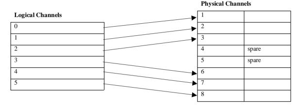
Noisy channels can be adapted out of the sequence by 'channel swapping', i.e. swapping a good spare channel for a noisy channel. For example, swapping physical channels 1 and 3 gives:
