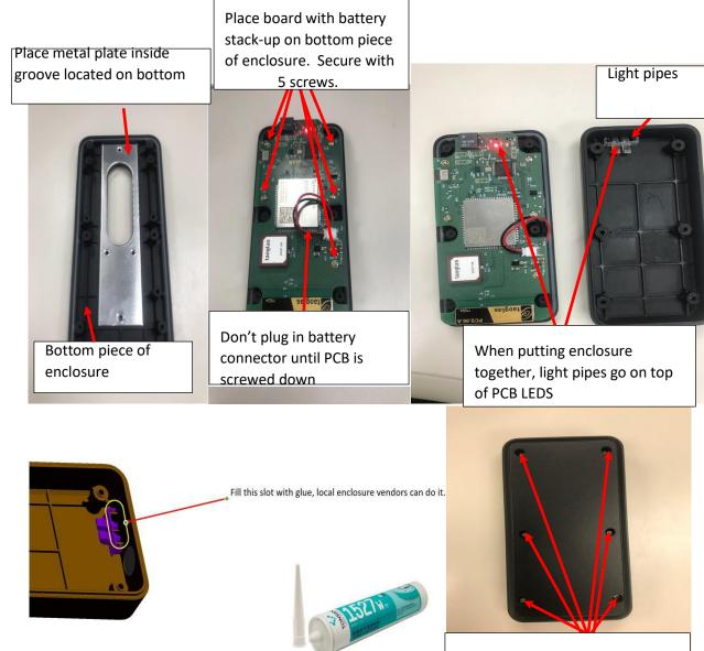
Use 6 of the same screws as used for PCB to secure enclosure
