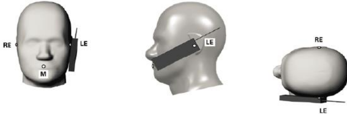
Fig. 11.3 Illustration for Cheek Position
