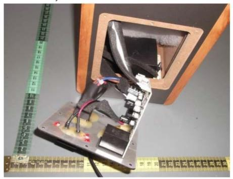
M/N: EDF100035: the power board is mounted on the rear panel and the PCB motherboard is mounted horizontally
