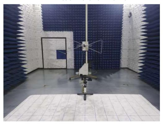
RADIATED EMISSION TEST SETUP ABOVE 1GHz
