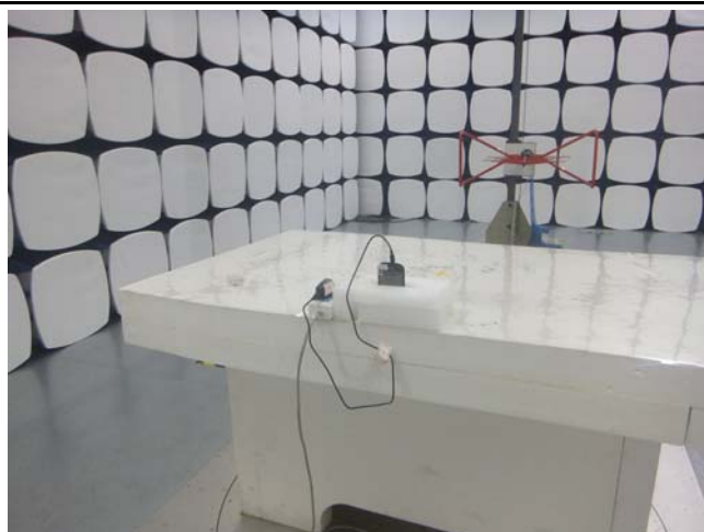
Conducted Emissions Test Setup Front View
