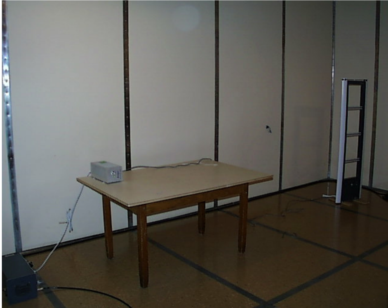
Photo 9 – Strata PX w/TR4024/22 Control Board Conducted Emissions Test Setup
