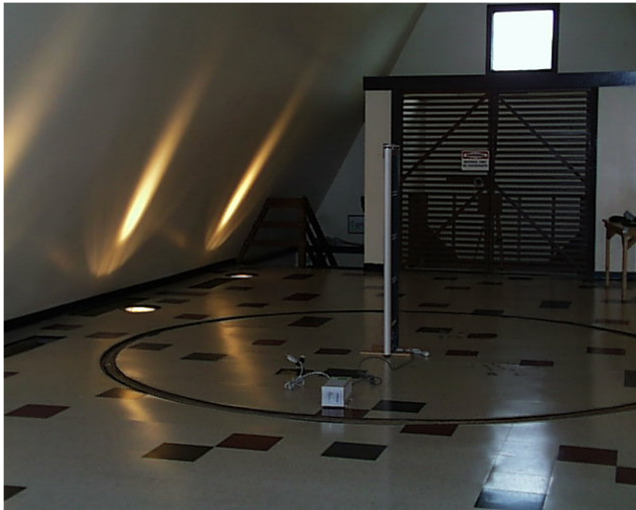
Photo 4 -- Strata PX w/TR4024/22 Control Board Radiated Emissions Test Setup -- Rear View
