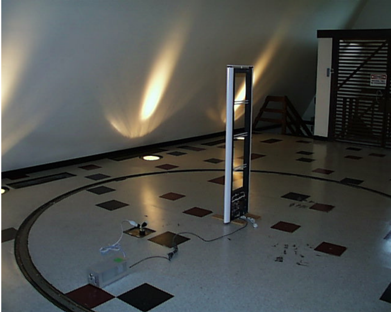
Photo 5 - Strata PX w/TR4024/22 Control Board Radiated Emissions Test Setup – Side View
