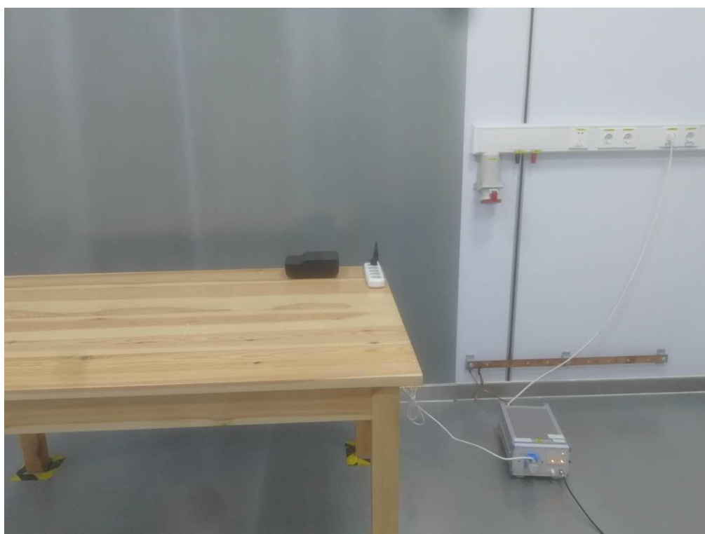
Fig. 4 Power line conducted emission setup photo
