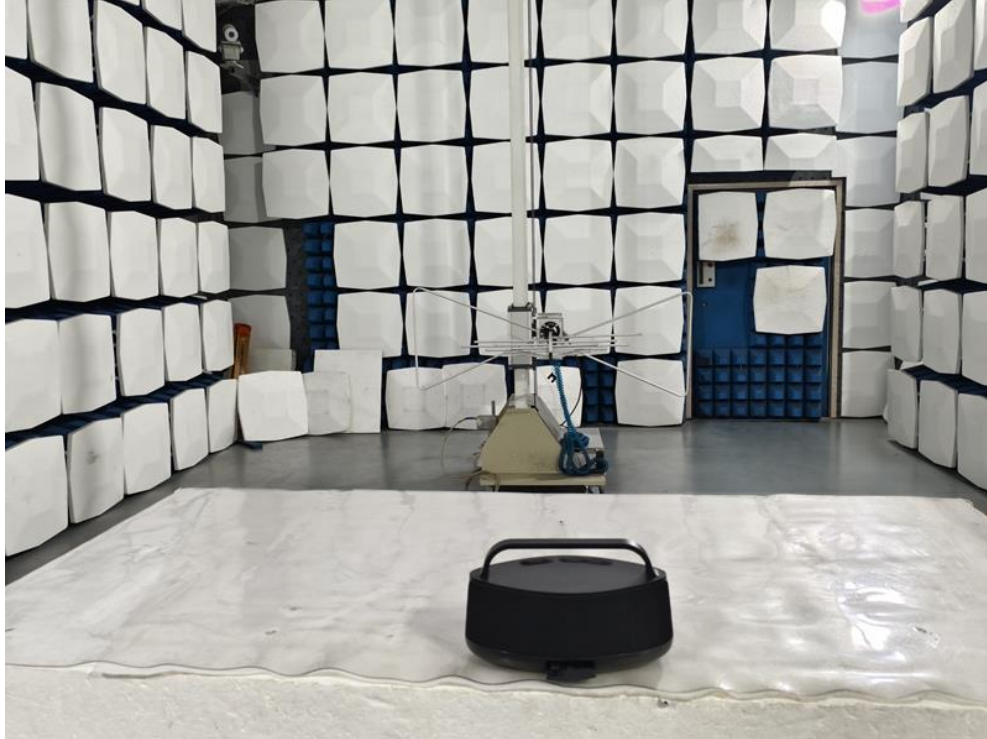
Radiated Emission Test Setup:
