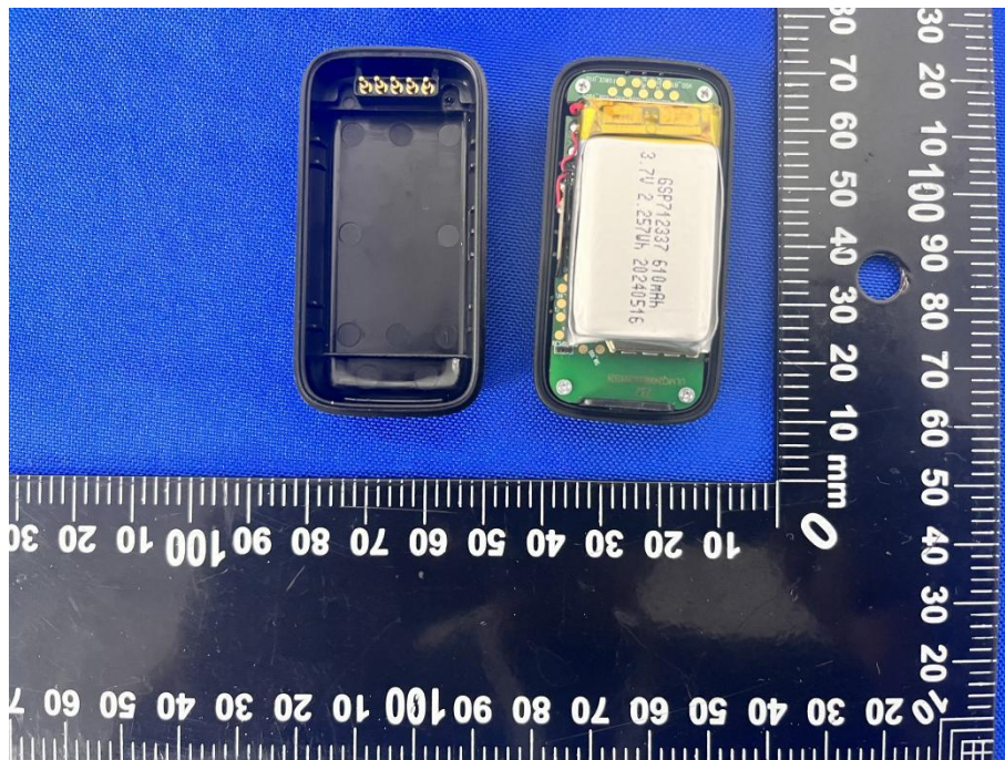
EUT UNCOVER VIEW 1(built-in GPS)
