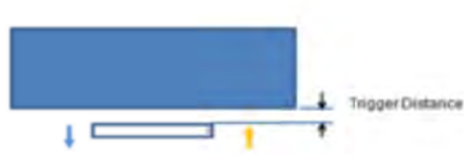
Picture : Proximity sensor triggering distances assessment (Back/front side)
