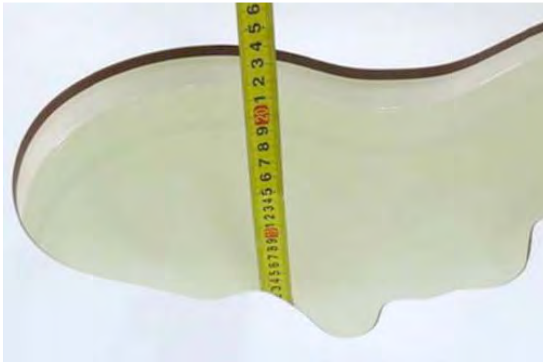
Picture 3: liquid depth in the head Phantom
