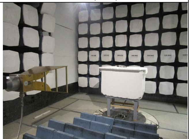
Radiated Emissions (>1GHz) – Rear View
