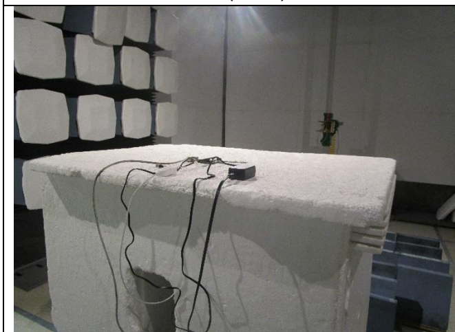
Radiated Emissions (>1GHz) – Front View
