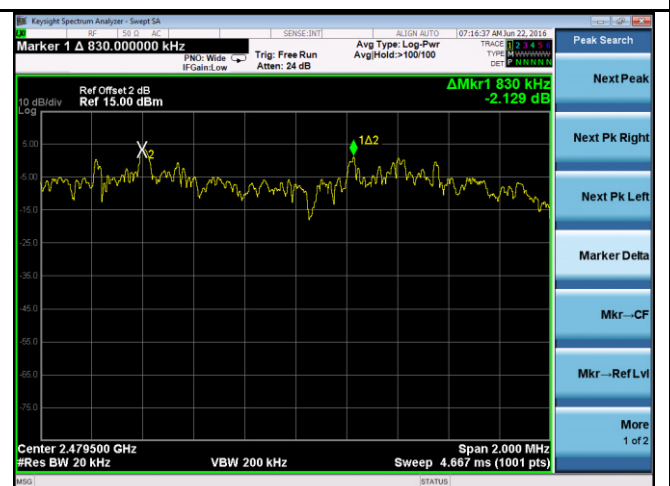
Channel Separation-EDR 2480MHz
