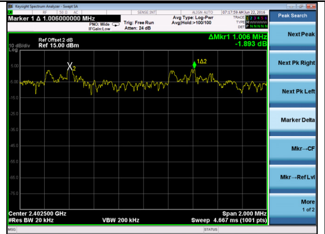
Channel Separation-EDR 2402MHz
