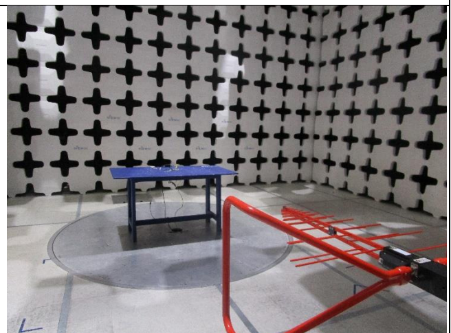
Radiated Emissions (<1GHz) – Rear View
