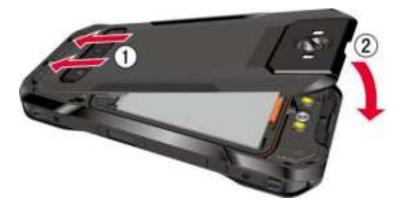
**NOTE:** The back cover will not close properly unless the battery latch is in the locked position.
