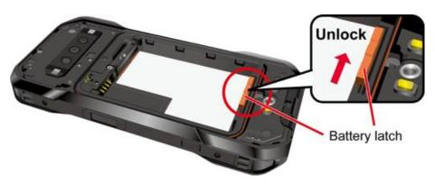
4. Insert the battery, making sure to align the gold contacts (1). Press down gently to secure the battery (2).
