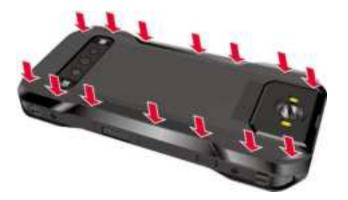
8. Using a coin, rotate the back cover screw to secure it. Do not overtighten.
