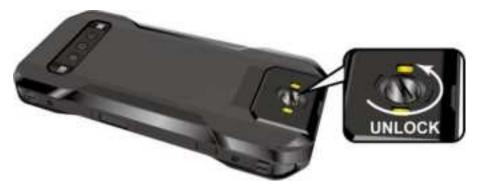
**NOTE:** The back cover screw is permanently mounted on the cover and cannot be removed.
