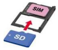
**NOTE:** If you need to reinstall your SIM card, remove the original SIM card from the tray and place your new SIM card into the tray with the gold contacts facing down as shown.
