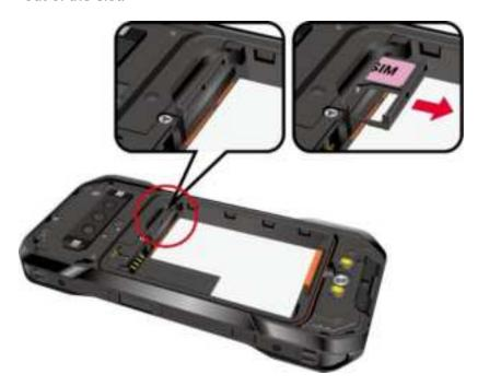
3. Put the tray onto a flat surface and place a microSD card into the tray. Ensure the gold contacts are facing down as shown.
