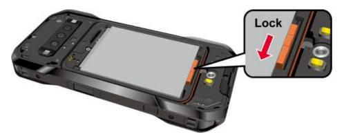
6. Insert the top edge of the back cover into place first before pressing the rest of the cover down.
