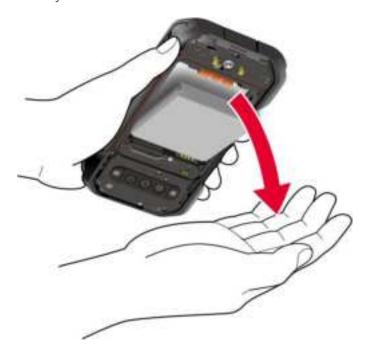
**CAUTION!** Do not use screwdrivers or other tools when removing the battery in order to avoid damage.
