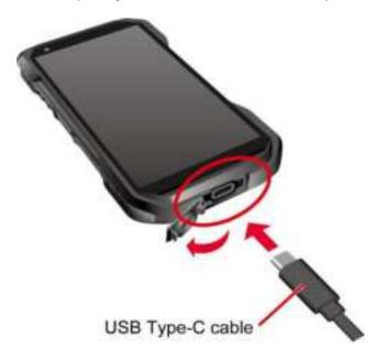
**IMPORTANT:** Only insert a USB Type-C connector into the phone's USB/Charger port.
