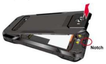
3. Unlock the battery latch by sliding it in the direction indicated by the arrow in the picture below.
