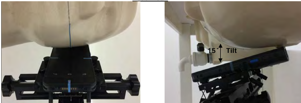
Fig.6 Left Head Section / Ear-Tilt Position(15°)
