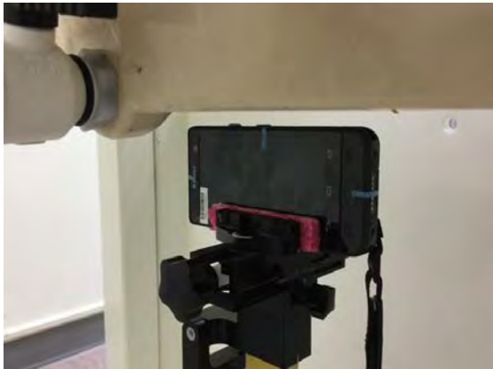
Fig.11 EUT Right side to flat phantom
