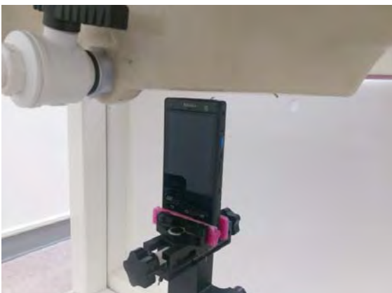
Fig.14 EUT Top side to flat phantom
