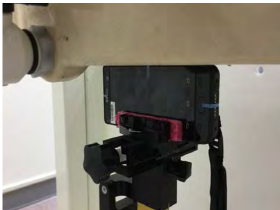
Fig.18 EUT Right side to flat phantom
