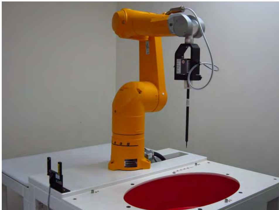
Fig.1 Photograph of the SAR measurement system
