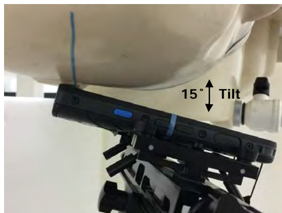
Fig.4 Right Head Section / Ear-Tilt Position(15°)
