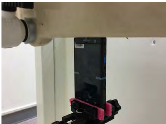
Fig.17 EUT Top side to flat phantom
