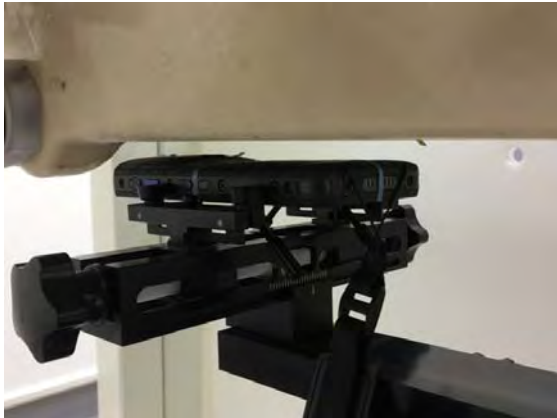
Fig.10 EUT Back side to flat phantom
