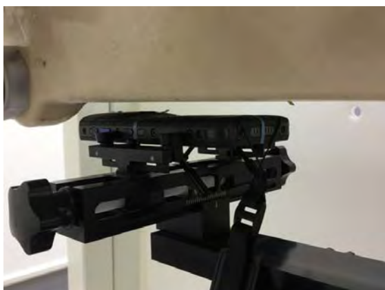
Fig.8 EUT Back side to flat phantom
