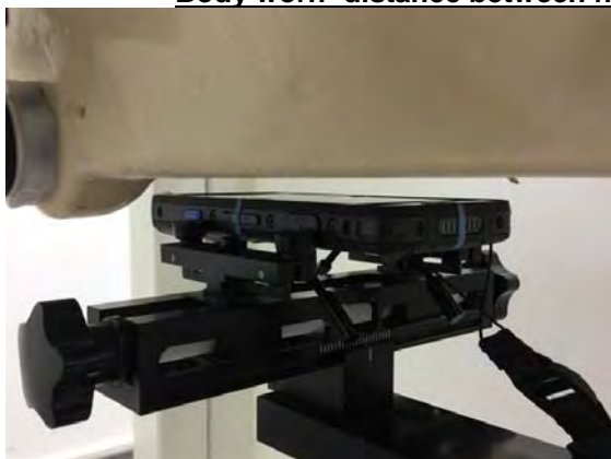
Fig.7 EUT Front side to flat phantom
