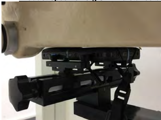
Fig.15 EUT Back side to flat phantom
