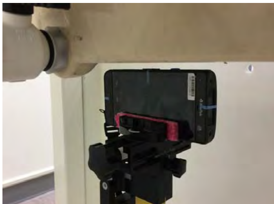
Fig.12 EUT Left side to flat phantom
