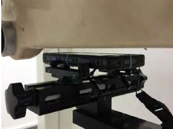
Fig.9 EUT Front side to flat phantom
