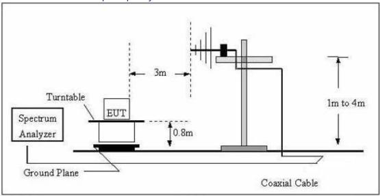
(C) Radiated Emission Test-Up Frequency Above 1GHz
