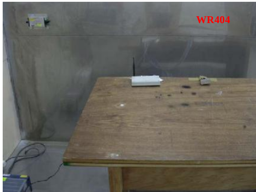
Photo 2: Conducted Emission Test Set-up
