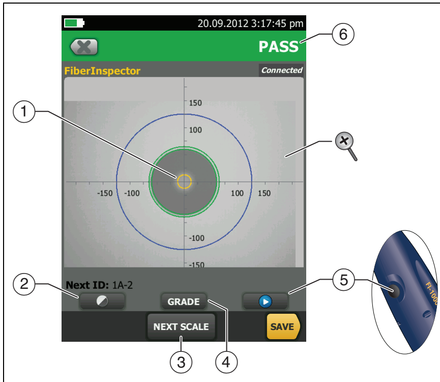
Figure 38. FiberInspector Image with Manual Grading Selected
