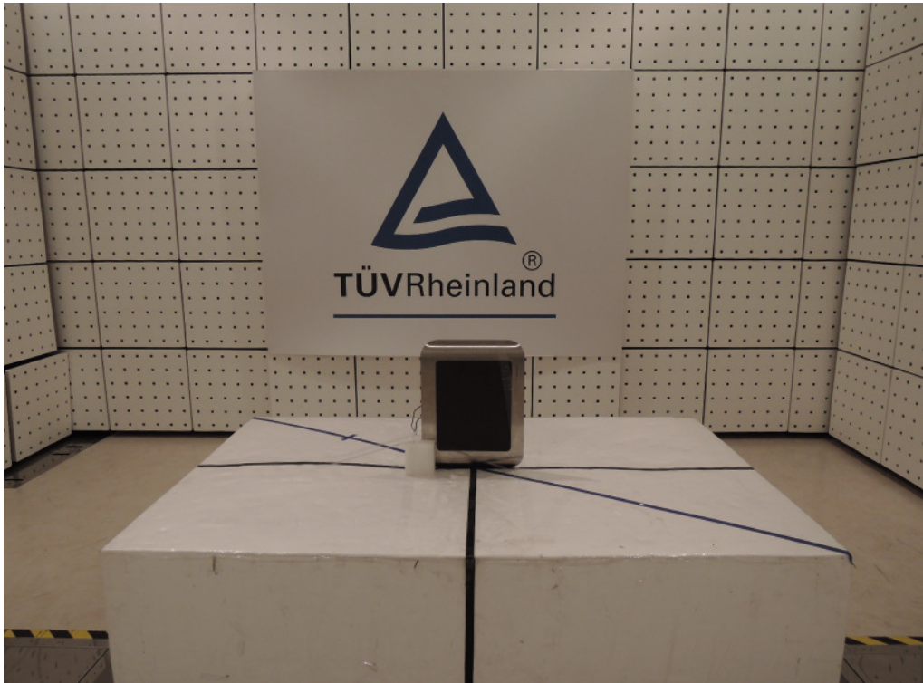
Photograph 1: Set-up for Spurious Emissions TX (Front View)
