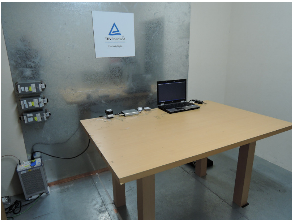
Photograph 5: Set-up for Mains Conducted testing Front
