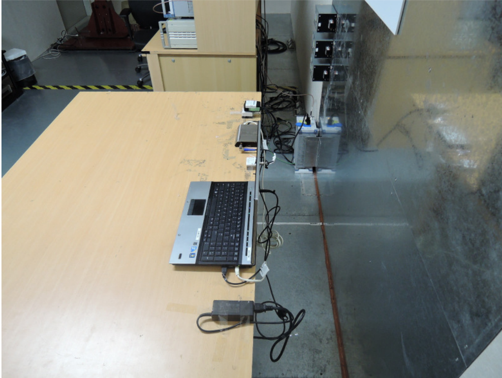
Photograph 4: Set-up for for Mains Conducted testing Back
