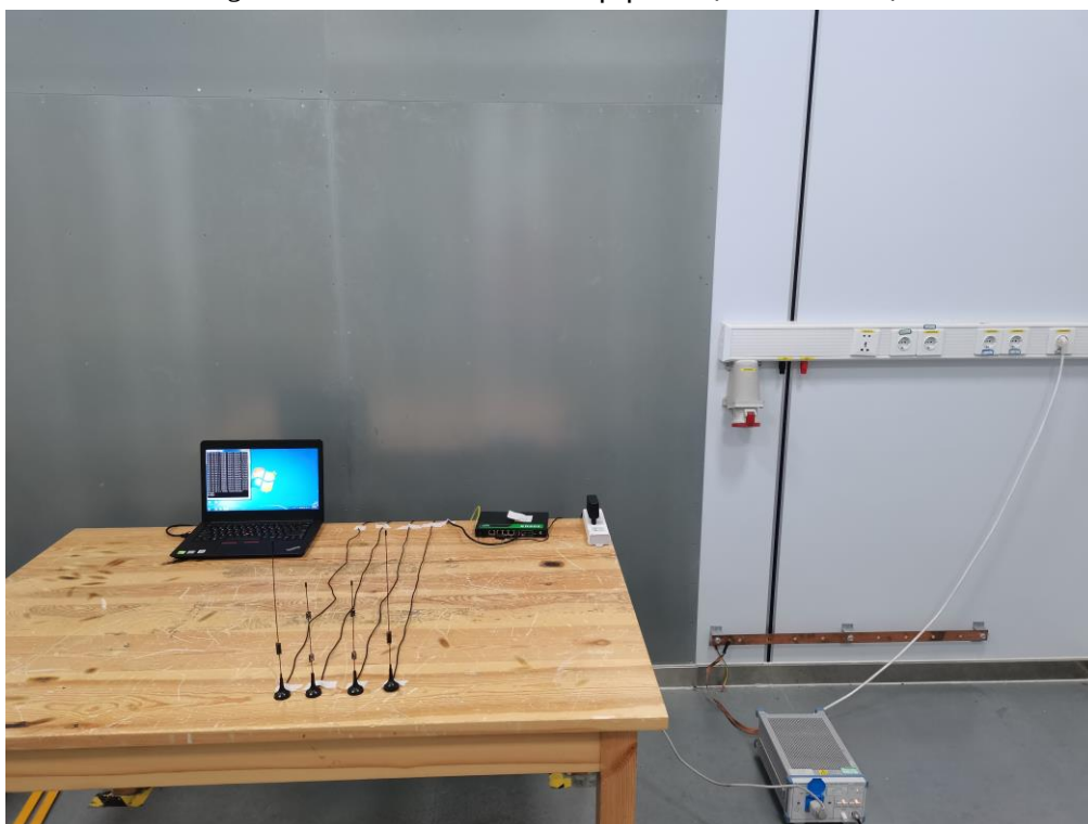
Fig. 4 Power line conducted emission setup photo
