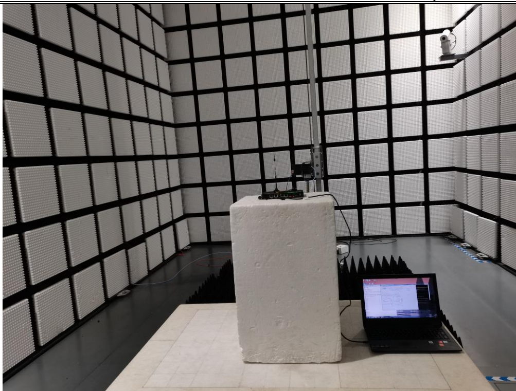
Fig. 3 Radiated emission setup photo(Above 1GHz)
