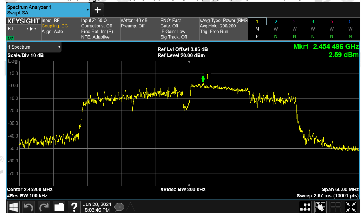
Band Edge NVNT be40 106+26RU Index 55+13 2452MHz Ant2 Emission
