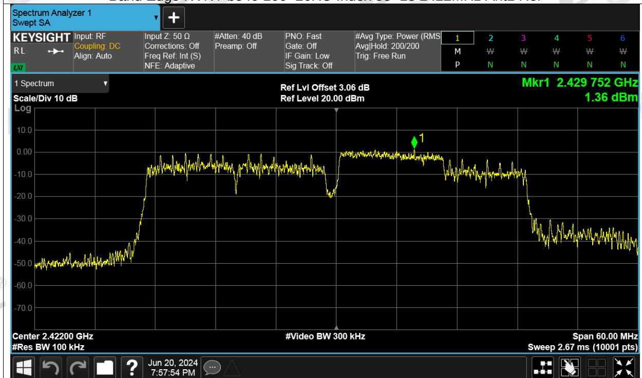
Band Edge NVNT be40 106+26RU Index 55+13 2422MHz Ant1 Emission
