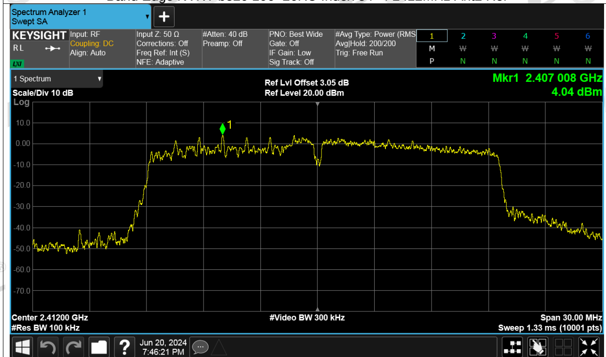
Band Edge NVNT be20 106+26RU Index 54+4 2412MHz Ant2 Emission
