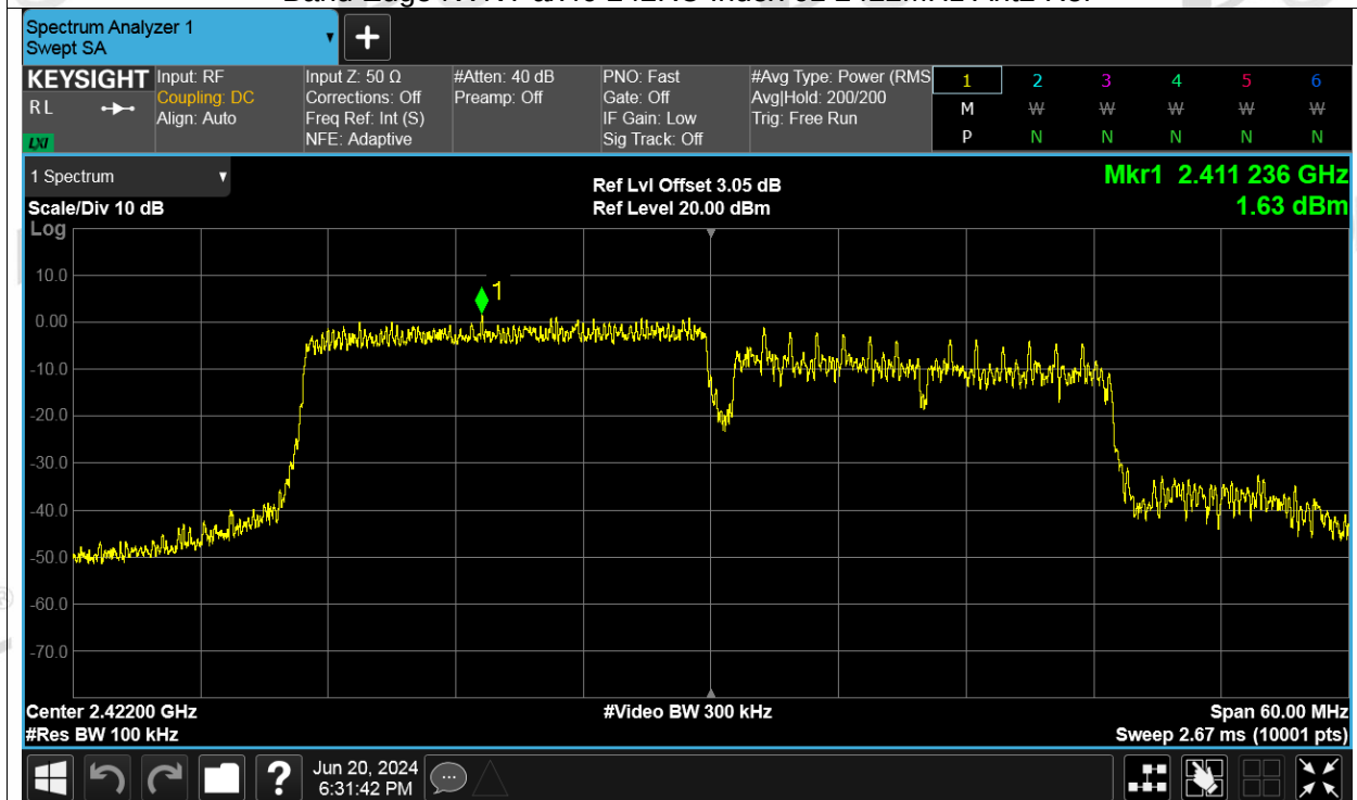
Band Edge NVNT ax40 242RU Index 61 2422MHz Ant2 Emission
