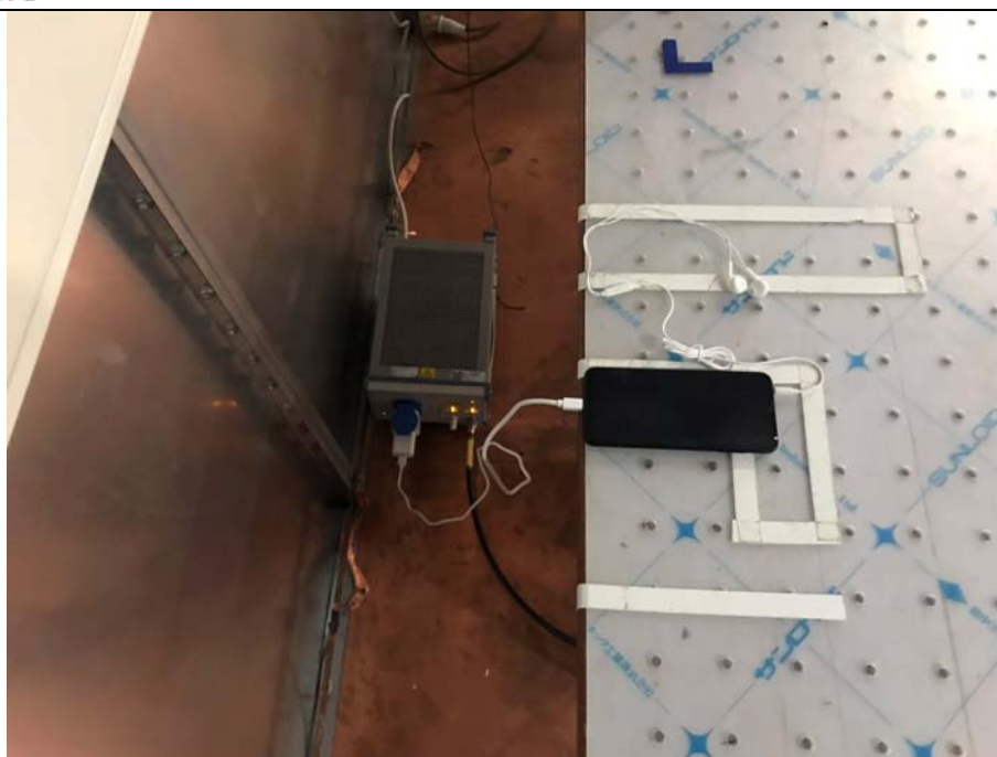
Conducted Emissions Test Setup (with charger)
