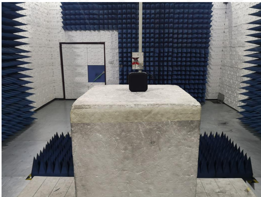
RADIATED EMISSION TEST SETUP ABOVE 1GHZ
